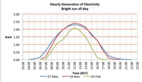
Monitoring of the PV system has enabled adjustments to be made to lifestyle and energy use to get the most from the renewable energy generated. Appliances are used when the PV system is generating and in sequence, not simultaneously. New appliances (when needed) draw relatively low levels of power (within the capacity of the PV system) or have some capacity to store energy.
